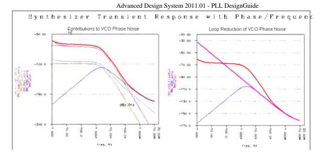
The graph on the left displays the individual noise source's contributions and the graph on the right shows the overall noise performance of the PLL.
