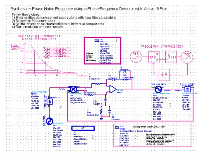
The phase noise characteristics of each component should be set on each subcircuit block. The F and L parameters that describe the noise versus frequency characteristics are depicted in the schematic.
