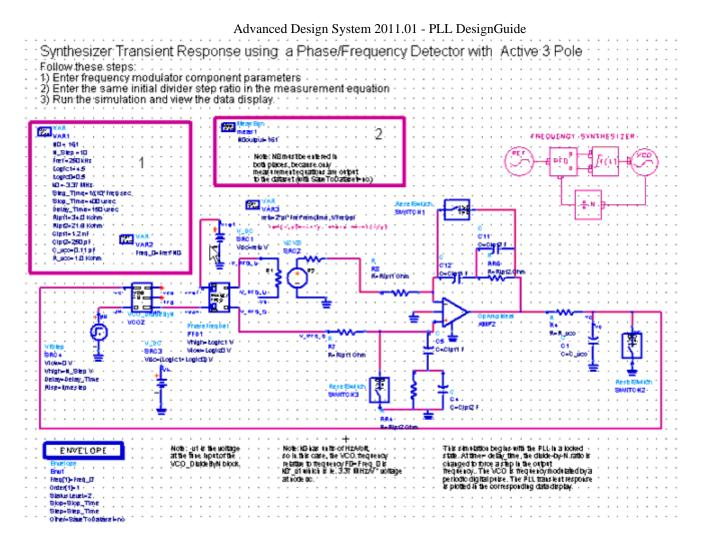
The loop filter parameters derived from the Loop Frequency response need to be entered into this schematic, along with the VCO and Phase Detector constants. The transient response requires additional parameters such as the Reference Frequency and the stop and delay time, as well as the Divider Ratio step change.
