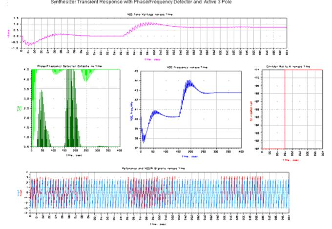
Synthesizer Transient Response with Phase/Frequency Detector and Active 3 Pole
