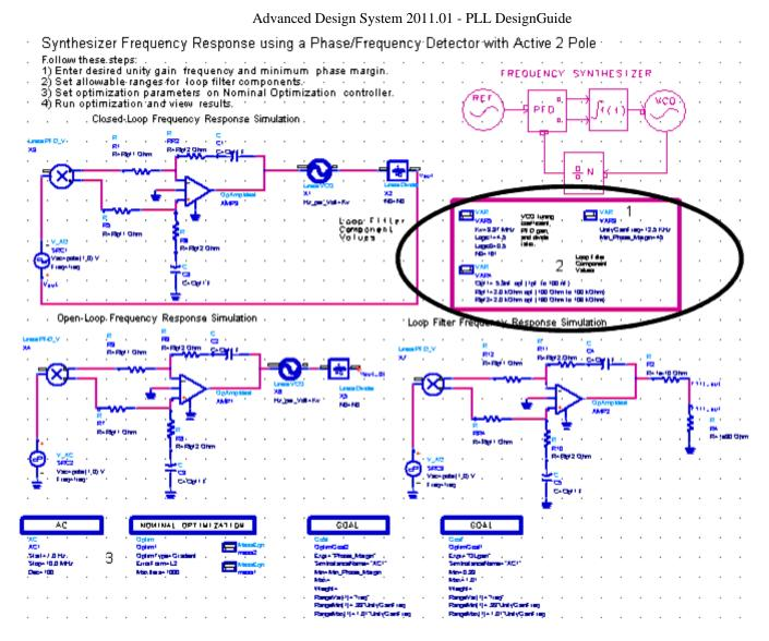
In the data display results shown here, the resultant Phase Margin and Unity Gain Frequency are displayed, along with the optimized loop filter parameters. If the objectives have not been met, you should adjust the loop filter parameters to alter the initial conditions of the optimization and re-run the simulation.
